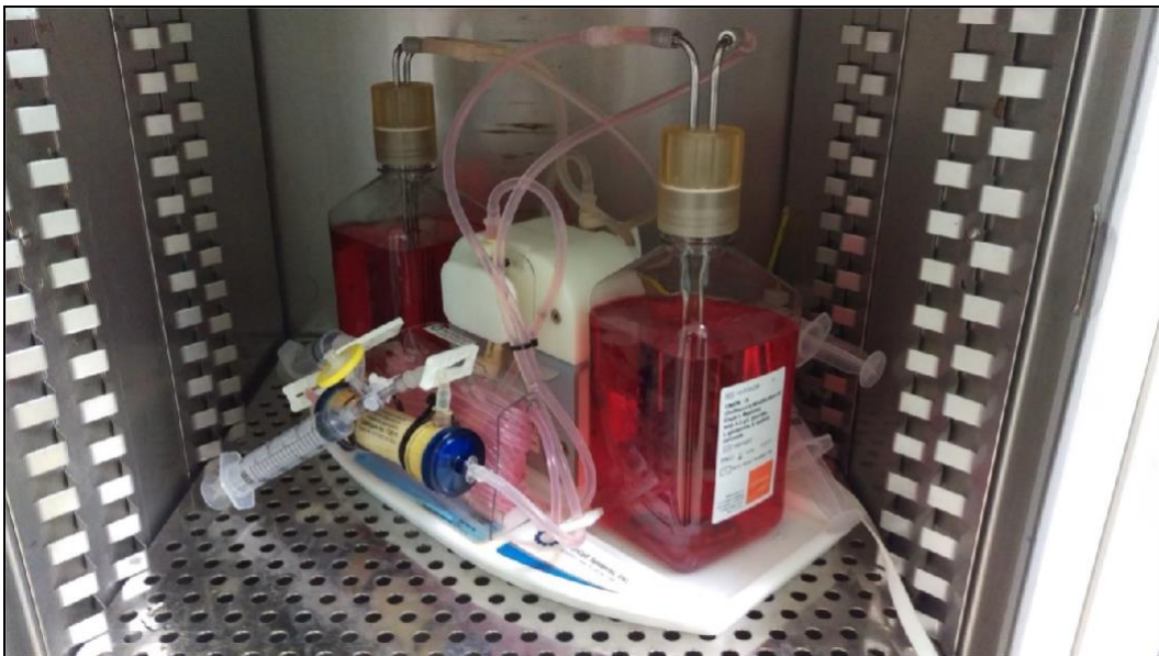
Figure 9: The hollow fiber bioreactor fits inside a standard CO 2 incubator. Temperature and gas are controlled by the conditions of the incubator. Reduced handling time and no cell passing reduces the time the cells are outside of the incubator.
