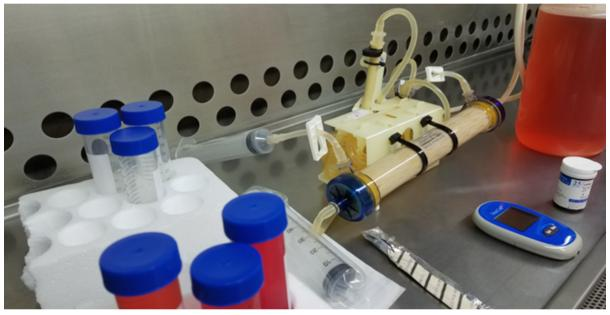
Figure 3: FiberCell Systems' 3D Bioreactor (C2018 Large Cartridge) with Harvests.
