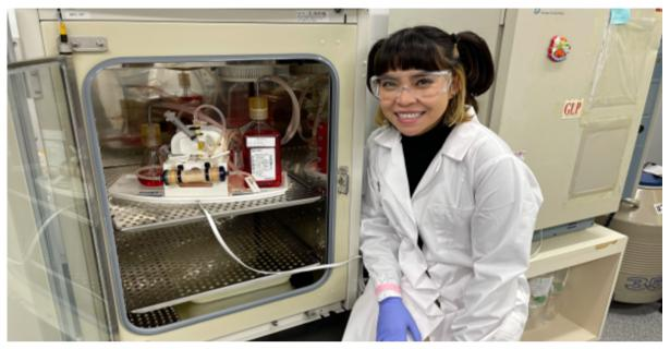
Figure 2: FiberCell Systems' 3D Hollow Fiber Bioreactor with Duet Pump in an Incubator.
