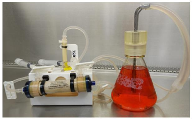
Figure 5: FiberCell Systems's 3D Bioreactor (C2011 Medium Cartridge) with Media Bottle.
