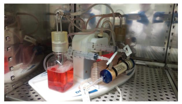
Figure 1: FiberCell Systems' 3D Hollow Fiber Bioreactor with Duet Pump in an Incubator.
