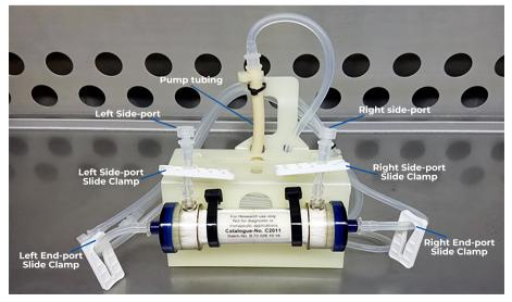
Figure 4: C2011 medium cartridge with parts identified.
