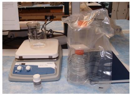
Figure 25: Materials required for rehydration of CDM HD.
