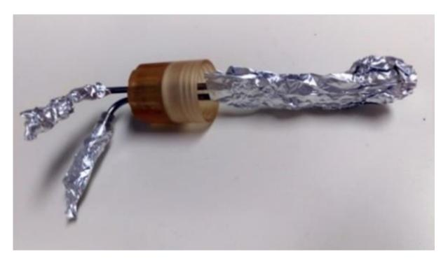
Figure 13: Aluminum foil protects the exposed parts of the reservoir cap. Once placed in autoclave bag the reservoir is ready to be autoclaved. Place the reservoir cap tubing on the hose barbs of the cap prior to autoclaving.
