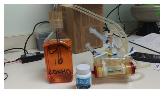
Figure 12: FiberCell System's Chemically Defined Serum Replacement for High-Density Culture (CDM HD).
