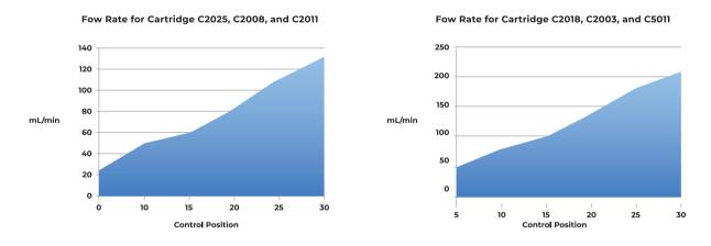
Figure 35: Duet flow rates vs. control knob position.
