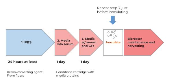
Figure 15: Block diagram of steps involved in setting up and seeding a cartridge.
