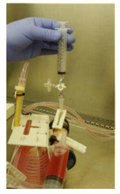
Figure 19: The Use of a 3-Way Stopcock and a Sterile Filter in Harvesting.
