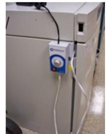
Figure 33: Thin cord for power fits in between incubator door.
