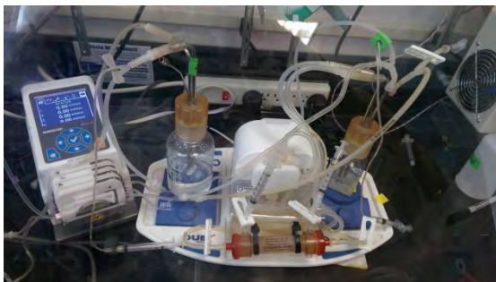
Figure 11: The hollow fiber infection model can be set up in an anaerobic chamber to control gas composition.
