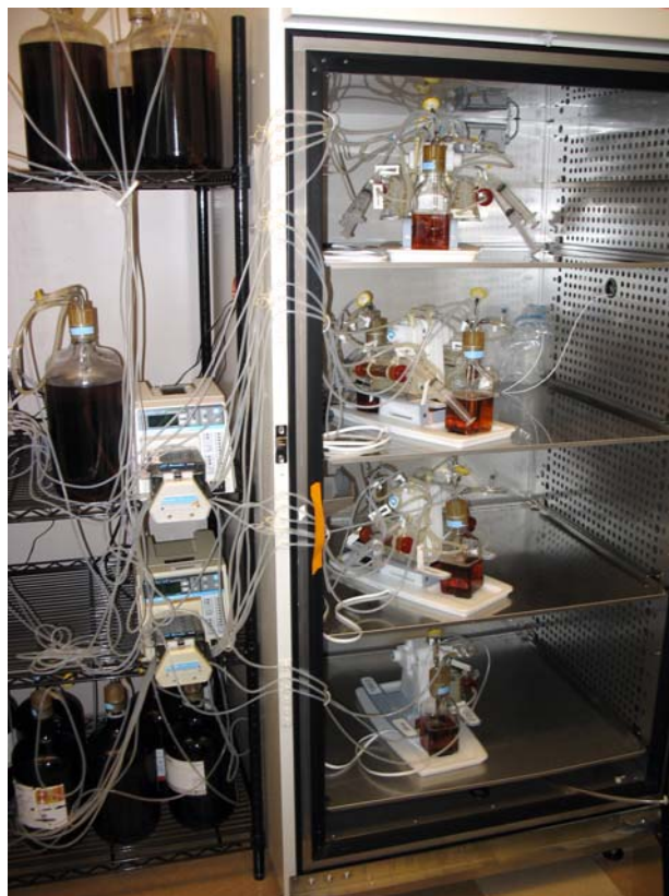
Example of the hollow fiber bioreactor cartridge setup. Note the large volume of diluent on the outside of the incubator and peristaltic pumps for controlled addition of diluent.
