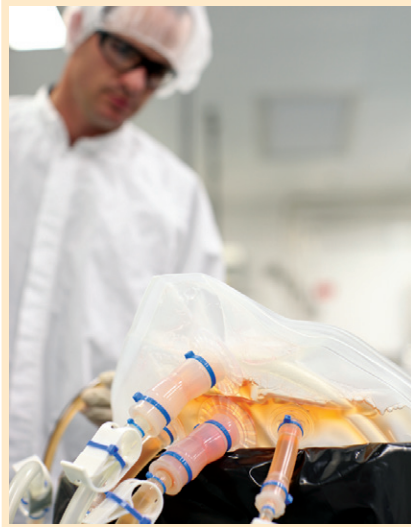
Photo 5: A Thermo Scientific BioProcess Container bag is filled with perfusion culture medium.
