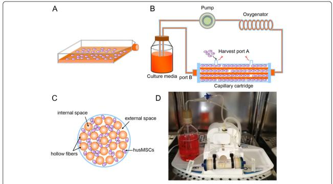
**Fig. 1** Schematic and photograph of the 2D and 3D culture system. **a** The schematic of conventional 2D flask. **b** The general schematic of the hollow fiber bioreactor-based 3D culture system. The system was composed of a pulsatile perfusion pump, an oxygenator, a cartridge containing thousands of hollow fibers, a bottle of culture medium, and the connecting tube. **c** A general schematic of cross-sectional view through the bioreactor. **d** The photograph of our 3D culture system
