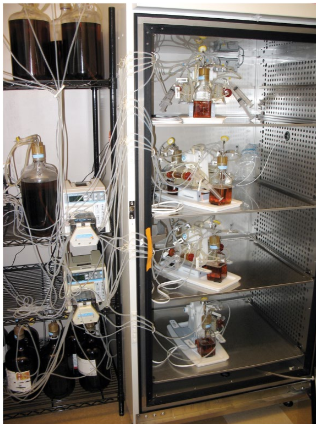
Figure 14.8 Example of a set-up to run multiple cartridges and multiple assays simultaneously. The closed nature of the system permits different experiments to be run in the same incubator.
