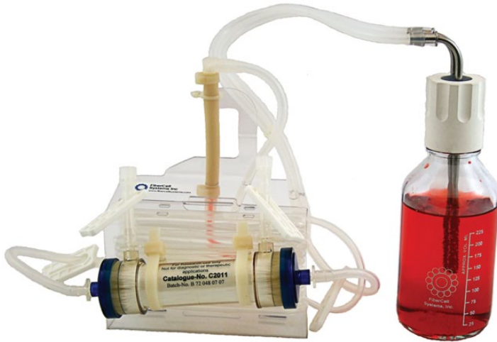
Figure 14.1 Hollow fibre cartridge A hollow fibre cartridge represents a single-use, bio-safe closed system for culturing cells, bacteria and viruses. The standard sized cartridge has an extracapillary space volume of 20 mL and 3000 cm 2 of area.
