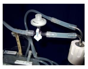
the polycarbonate luers on the stopcock. You may want to consider a small drop of adhesive (such as Krazy Glue®) to make certain that the connection does not come loose. After the stop cock is in place simple place the sterile filter over the middle luer connection. This provides a sterile barrier between the medium and the sampling syringe. Take the luer cap and use it to cover the external fitting on the filter. You should plan on replacing the filter at least once every 30 days.
