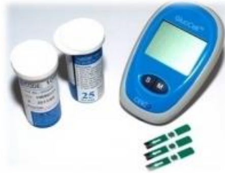
GlucCell classical media glucose monitor or chemical analyzer for measuring glucose. Diabetic test strips will not work with classical media.
