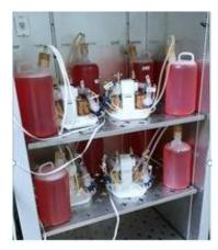
A hollow fiber bioreactor is very compact, easy to install, easily scalable and very affordable. Left, is a photo of a set consisting of 4 pumps and 8 hollow fiber cartridges capable of generating 2 grams of mAb per week with a good hybridoma, or 400 mg per week of recombinant protein.
