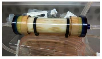
Operation of a HF bioreactor begins by seeding a prepared cartridge with either suspension or harvested adherent cells. The hollow fiber module is connected to an external reservoir and the medium recirculated from the reservoir through the cartridge. The FiberCell Duet pump provides high rates of flow (80-160 mL/minute) using a positive pressure displacement pump mechanism
