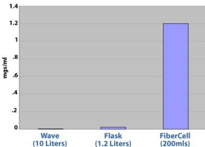
**Figure 4: Antibody yield per 10 L of medium consumed, total harvested antibody concentration prior to purification.** Note the extremely high concentration of antibody in the FiberCell Systems hollow fiber bioreactor cartridge. 200 mL of harvested supernatant was equivalent to 10 L of culture supernatant from the other systems again reflecting the 50 X higher concentration of antibody generated in the FiberCell Systems bioreactor cartridge.
