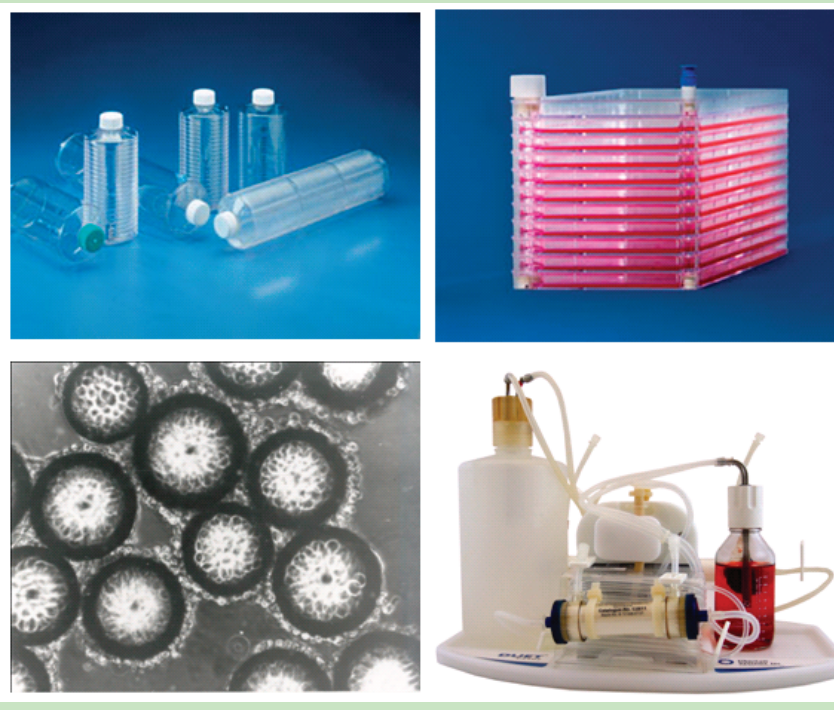
Figure 2: Adherent cell vaccine production formats; (A) Roller bottles come with standard or expanded surfaces and a range of surface areas; pictured are Thermo Scientific Nunc In Vitro PETG brand (Thermo Fisher Scientific). (B) Stacked-array flasks have been optimized for industrial-scale production of vaccines; pictured is a Thermo Scientific Nunc 10-tray Cell Factory system (Thermo Fisher Scientific). (C) Microcarriers have surfaces that support cell attachment and growth; pictured are cells on Hillex II microcarriers (SoloHill Engineering). (D) Hollow-fiber bioreactors provide scalable, continuous-processing virus production; pictured is a FiberCell Duet system (FiberCell Systems Inc.).
