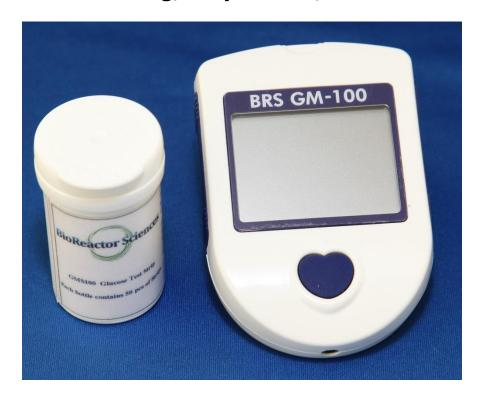
The GM100 Glucose Monitoring System is specifically designed to quantitatively measure the glucose concentration in microbial and cell culture bioprocessing applications. Disposable test strips and its compact size enable operation of the GM-100 Glucose Monitoring System in a biosafety cabinet, eliminating risk of contamination from biohazardous samples.
