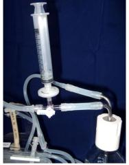
the polycarbonate luers on the stopcock. You may want to consider a small drop of adhesive (such as Krazy Glue®) to make certain that the connection does not come loose. After the stop cock is in place simple place the sterile filter over the middle luer connection. This provides a sterile barrier between the medium and the sampling syringe. Take the luer cap and use it to cover the external fitting on the filter. You should plan on replacing the filter at least once every 30 days.
