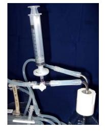
certain that the connection does not come loose. After the stop cock is in place simple place the sterile filter over the middle luer connection. This provides a sterile barrier between the medium and the sampling syringe. Take the luer cap and use it to cover the external fitting on the filter. You should plan on replacing the filter at least once every 30 days.
